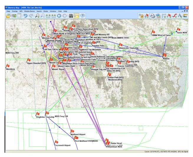
The purple lines are 'reference lines'. When parts of the transcript say that, for example, he is '36nm north of Singleton on the Mount Sandon / Singleton track' there is a line drawn between the Singleton NDB navigation aid, and the Mount Sandon VOR navigation aid. Then, a point 36nm north of Singleton on that line is marked.
