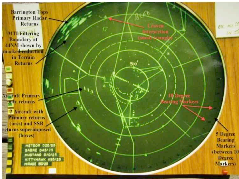
Figure 49: Williamtown SURAD PPI. Although this photo is of an approach PPI rather than the tower PPI used during the VH-MDX accident, almost everything except for the size was the same. The tower PPI was a little smaller (17") than the approach PPI (Photo: H. Howard c.1983).
