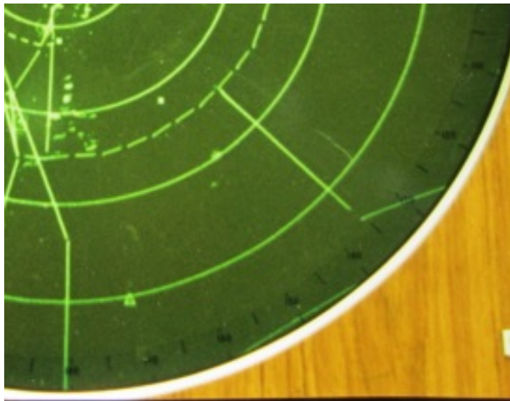
Figure 50: Williamtown SURAD approach PPI rose. This photo shows the compass rose with 5^\circ and 10^\circ marks and numeric values for each 10^\circ value. 10NM range rings are also visible. (Photo: H. Howard c.1983).
