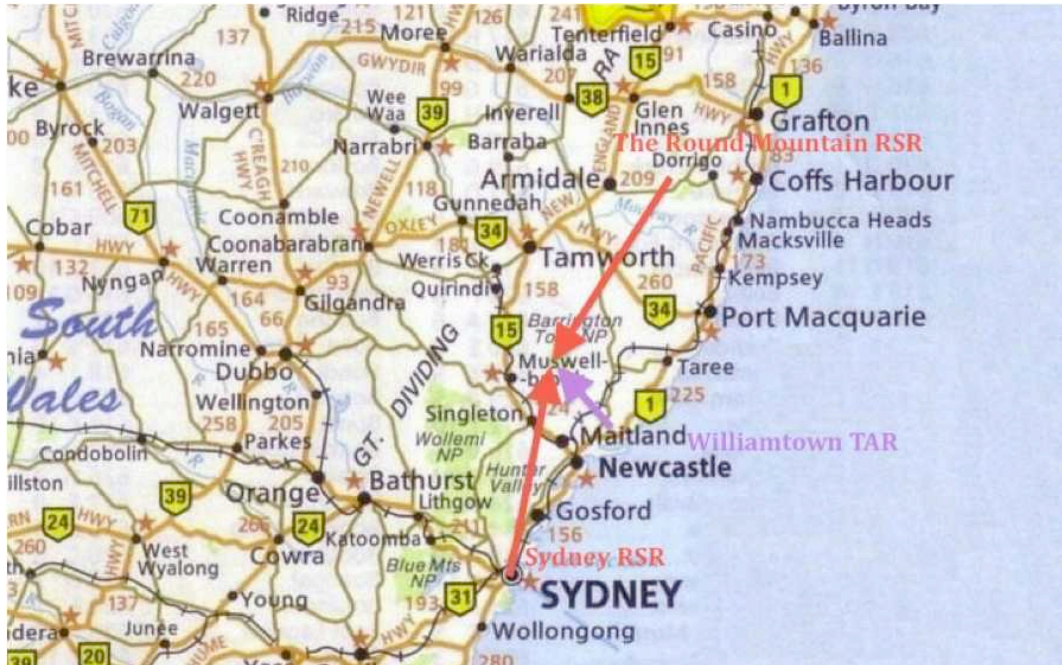
Figure 16: Relevant radar head locations. The Round Mountain RSR and Sydney RSR were operated by Sydney ATC (red arrows). Immediately obvious is how much closer to VH-MDX Williamtown TAR was. Despite this, as will be discussed only a single complete radar fix was obtained by Williamtown TAR (Base Map: Melway Publishing Pty Ltd 2014, additions: Glenn Strkalj 2014).
