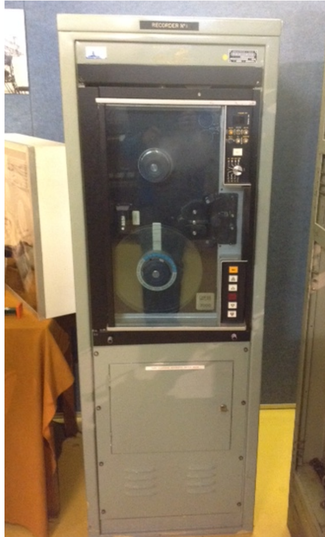
Figure 20: Radar Recorder unit. The unit is a SE7000 data recorder labeled 'Radar Recorder' (Image: Glenn Strkalj 2015).
