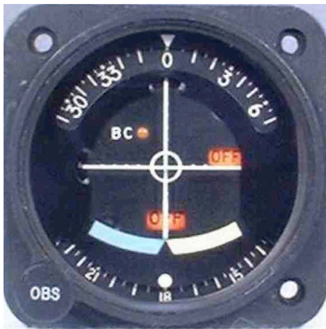
Figure 32: IN-525R VOR Omni Bearing Indicator (OBI). This indicator was listed in BASI archives as being fitted on board VH-MDX when delivered to Australia in 1977. Unlike the fixed card ADF, the OBI presents magnetic bearing information to the pilot. This simplifies obtaining magnetic bearing information to the pilot compared to the ADF. The knob on the bottom left is turned until the vertical needle is centered. The magnetic bearing is simply read off the top scale; in this case 000°M. A small ‘to/from’ indicator (not visible in the photo) indicates if the aircraft is positioned on the hemisphere that is going ‘to’ the indicated bearing (selected bearing is on the other side of the VOR ground station) or ‘from’ the selected bearing (selected bearing is on same side as the aircraft relative to the ground station). (Photo: Bennett Avionics 2001-2014).
