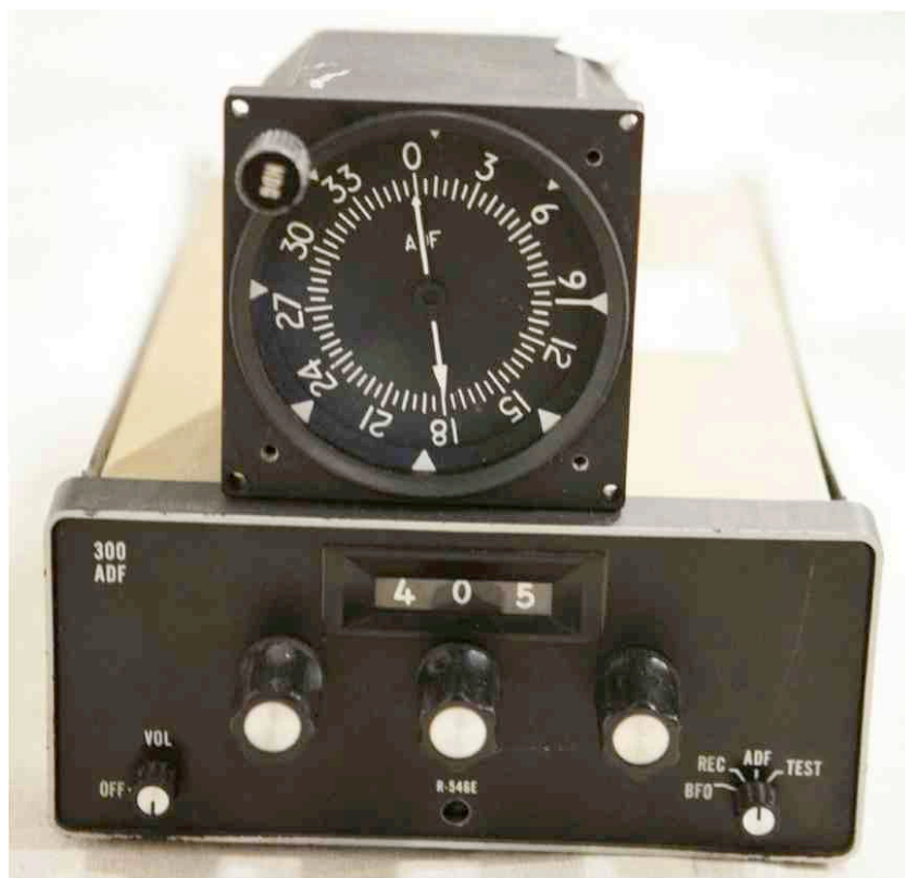
Figure 30: IN-346A fixed card ADF indicator and ARC R546E ADF receiver. These particular units were likely onboard VH-MDX during the accident. 'Fixed card' refers to the fact that the compass rose is not continually slaved to magnetic north as in some indicators. Despite this, the pilot is still able to manually rotate the card to any position. This is handy when transposing compass headings to the fixed card indicator in order to convert the displayed relative bearings to magnetic bearings.
