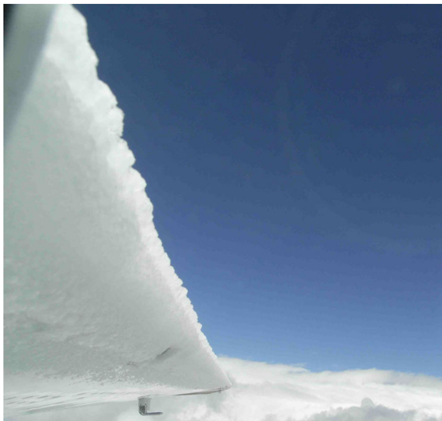
Figure 57: Icing accumulation: Cessna 210 wing leading edge. Significant ice has accumulated on the leading edge and immediately aft and underneath. The pilot's view from the Cessna 210 cockpit does not allow inspection of the critical upper surface of the wing. The effects of the rough and jagged ice on laminar airflow of the wing is readily predictable when viewing this photo. It can be seen why stall speed and drag increases. Additionally, the extra weight of the ice can be significant further burdening performance. The pitot tube under the wing is free of ice indicating that pitot heating was probably selected during this ice encounter.
