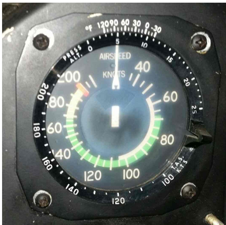
Figure 45: Cessna 210M Air Speed Indicator (ASI). It can be seen that reference to rounded off numbers would be simpler in turbulence. The beginning of the yellow band represents the speed at which a symmetrical 3000fpm gust would induce a load factor in excess of the aircraft's design load limit: Vno (Maximum structural cruising speed). Should a pilot control input be applied at the same time as a gust is experienced below 168KIAS, overstress is still possible as Vno only considers the gust . Maneuvering (Va) and Turbulence Penetration (Vb) speeds are not normally marked on the ASI but are normally placarded on the instrument panel. For the C-210M Va equals Vb and varies with weight being 119KIAS at MTOW. Va considers the effects on structure from only a single control input at one time in one control axis. Any of the following or combinations thereof, of simultaneous multiple axis and/or reversing control inputs and/or gusts will invalidate the protection of Va. The C-210M normally cruises at IAS's around 145KIAS: about 25knots above MTOW Va and 15 knots below Vno (Photo: N. McGlone 2015).
