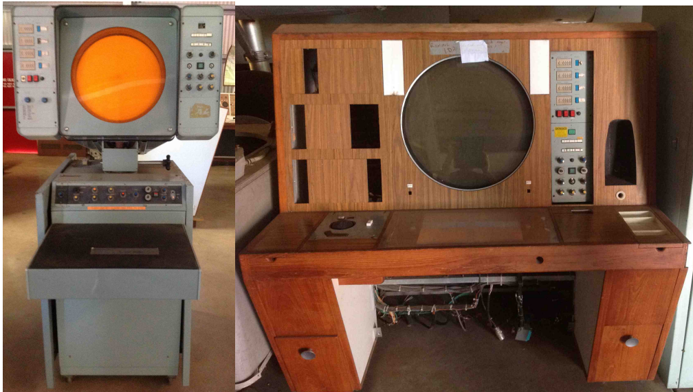
Figure 14: SURAD Maintenance PPI (left) and Approach PPI (right). (Photo: Glenn Strkalj 2014, access to SURAD PPI courtesy of The Australian Aviation Heritage Centre).
