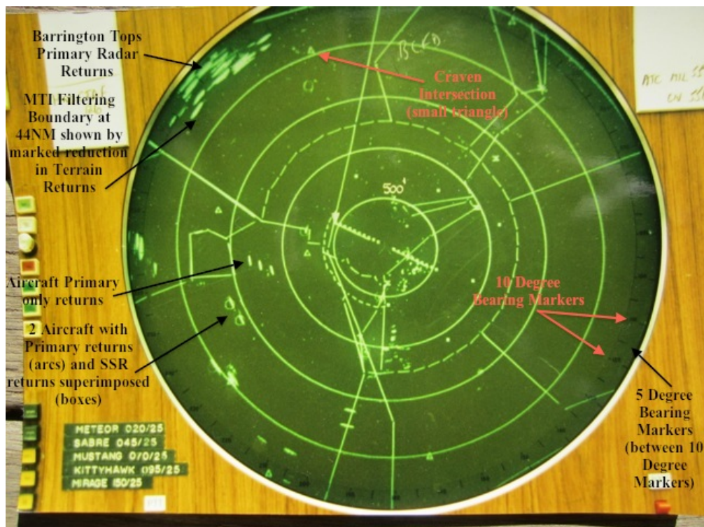
Figure 15: RAAF Williamtown Approach room SURAD PPI. North is at the top of the PPI. The compass rose on the circumference displays bearing in 10° increments with 5° markings in between. 10NM spaced rings are displayed to determine target range whilst airspace boundary markings and reporting points (small triangles) are also displayed. PSR returns show as arcs on the PPI with a good example of aircraft being at approximately 25NM west where three PSR returns are apparent. To the north-west from around 43NM are the permanent echo terrain returns of the Barrington Tops and the effects of MTI filtering can readily be seen with suppression of terrain occurring sharply from about 43NM and less. At approximately 32NM to the west-south-west are two PSR returns from aircraft that are also returning an SSR code as indicated by the symbols (circles) superimposed over the top. It can be seen from these two aircraft how SSR symbols overlay the PSR return. (Photo: H. Howard c.1983).
