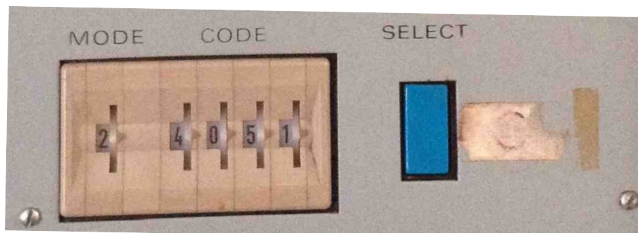
Figure 12: SSR symbol preset. Displayed SSR symbols could be allocated to a specific ATRBS mode code as preset by the thumbwheel switches shown. In this case aircraft squawking mode 2 code 4051 would be displayed by a circle (as drawn on the sticker to right) on the PPI when the 'Select' button was pushed to on. Note: mode A is also known as mode '3A' so, would be represented as mode '3' using the thumbwheel switches (Photo: Glenn Strkalj 2014, access to SURAD PPI courtesy of The Australian Aviation Heritage Centre).
