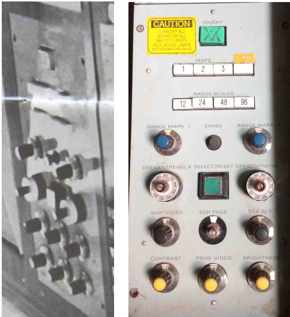
Figure 19: SURAD Tower PPI controls. Left photo is a zoom of the Williamtown Tower PPI control panel, the right photo a SURAD approach PPI control panel from Darwin SURAD. Both appear similar so, the Darwin SURAD panel can be used as a reference to determine controls (Left photo: H. Howard c.1983; Right photo: Glenn Strkalj 2014, access to SURAD PPI courtesy of The Australian Aviation Heritage Centre).
