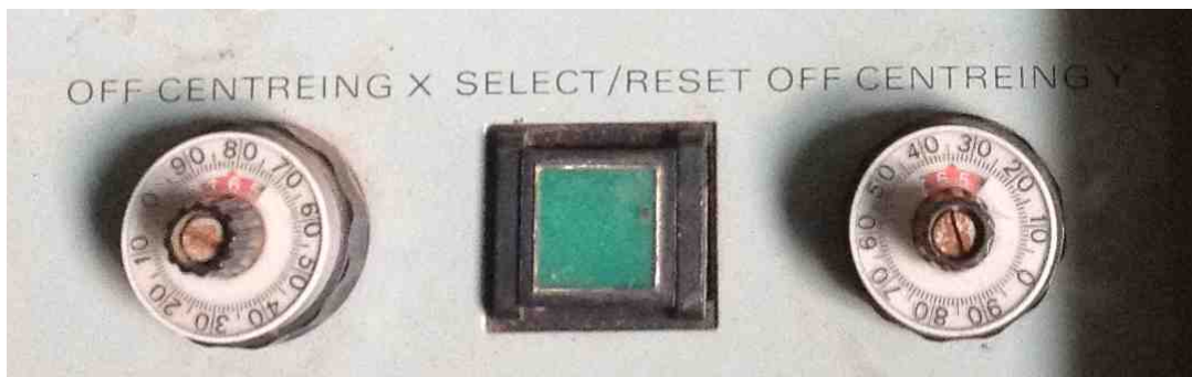
Figure 17: PPI offset controls. The displayed area on the PPI could be offset away from the radar head at origin position. Two controls were available to move the PPI origin position in both the X and Y-axis. The offset was then activated or cancelled by pressing the 'Select/Reset' button. (Photo: Glenn Strkalj 2014, access to SURAD PPI courtesy of The Australian Aviation Heritage Centre).
