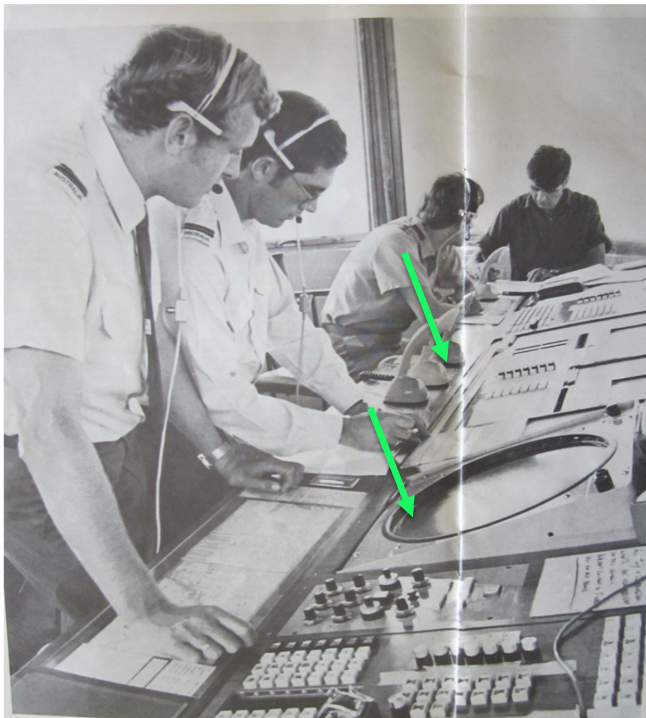
Figure 18: Williamtown control tower c.1970's. The SURAD Tower PPI is apparent albeit not the information displayed. It was reported that the angle of the PPI and low layout in the console resulted in poor ergonomics [5] . Specifically, head movements between looking outside, strips and the PPI was unnatural [5] . As the tower was situated south, sun glare from a rising or setting sun would restrict readability of radar returns on the PPI [5] . Accordingly, a metal shroud was incorporated to reduce glare on the PPI [4][5] . Note the locations of communication equipment and flight strips away from the PPI. The ATCO during the night of the accident would likely have operated between the two green arrows, the distance being estimated at around two meters [5] . The main procedural area was between the second ATCO from the foreground to the position of the far arrow [5] (Photo: H. Howard c.1970's).
