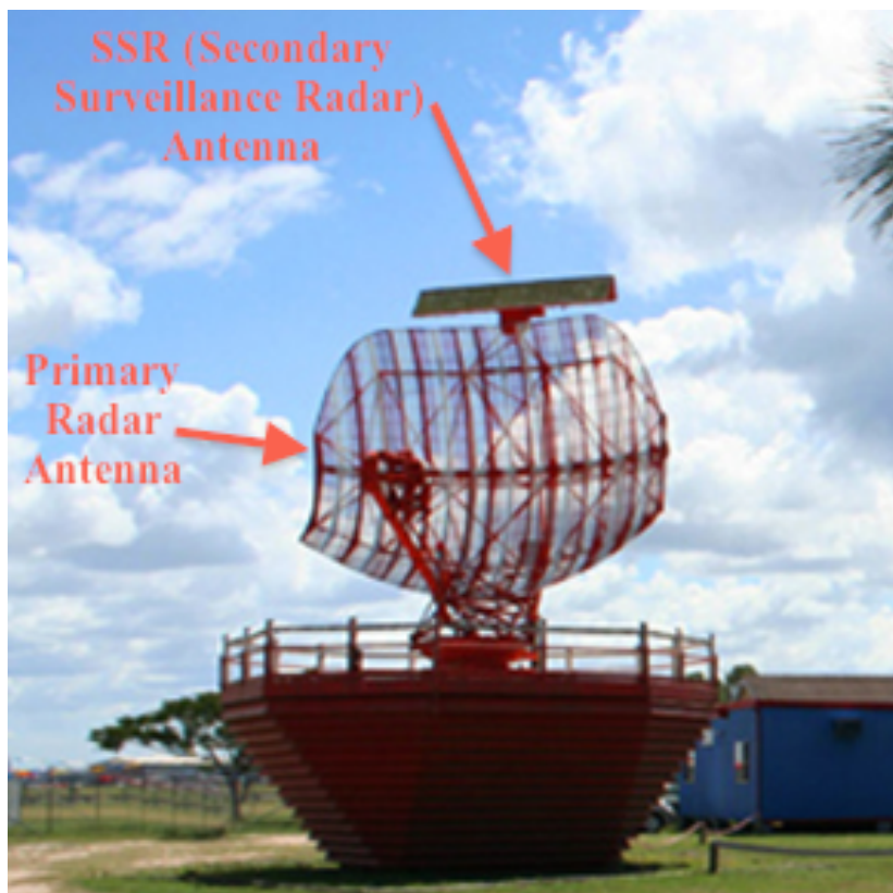
Figure 2: SURAD radar head. The main antenna or 'dish' services the PSR system and atop this is the SSR antenna. PSR is passive, relying on radio wave reflections from a target. SSR is active in that ground interrogator and aircraft transponder 'talk' to each other. The two systems, PSR and SSR are isolated systems other than sharing the same display screens (PPI's). The radar head would be mounted at the top of a steel tower to increase line of sight thus increasing range unlike this museum piece mounted on the ground. (Photo: Fighter World Aviation Museum 2014).
