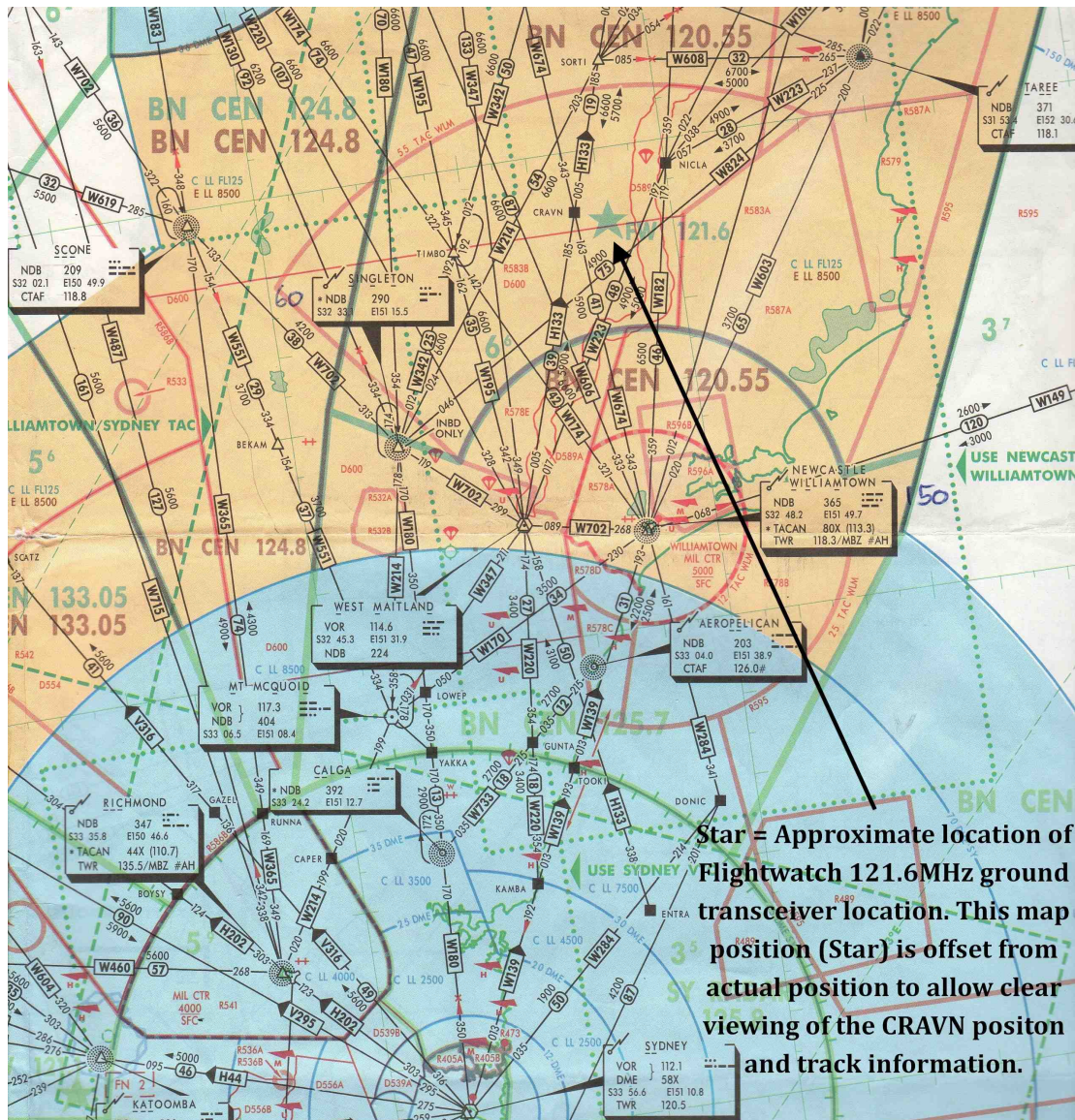
Figure 7: Enroute Chart Low 3, November 2001 [9] . The star indicates the approximate position of the Flightwatch 121.6MHz ground based transceiver. These stars are often offset from the actual ground station position to allow clarity in reading other more important information that in this case is the CRAVN position and associated bearing information. This chart confirms 121.6MHz as being used for FIS purposes in the Barrington area during 2001. It was unlikely the frequency was changed since 1981 to 2001 despite the callsign having changed (Chart: Aircservices Australia 2001, additions: Glenn Strkalj 2014).
