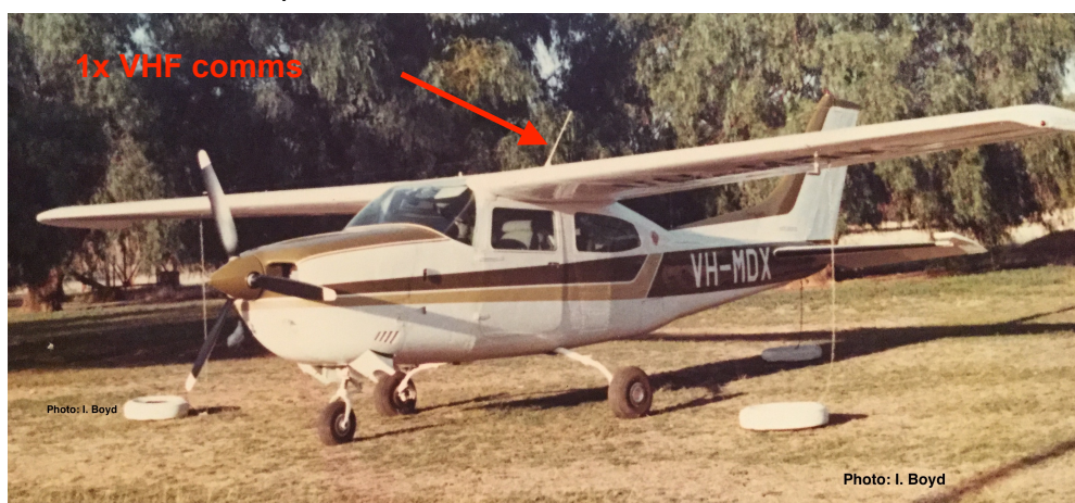
Figure 2: VH-MDX VHF Communication antennae position. Also visible are the VHF Nav antennas, HF Comm antenna and ELT(Electronic Location Beacon) antenna (Photo: I. Boyd c.late 1970's obtained by G. Strkalj 2017).
