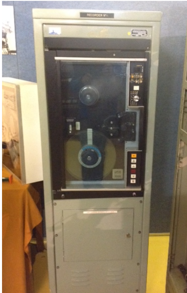
Figure 20: Radar Recorder unit. The unit is a SE7000 data recorder labeled 'Radar Recorder' (Image: Glenn Strkalj 2015).
