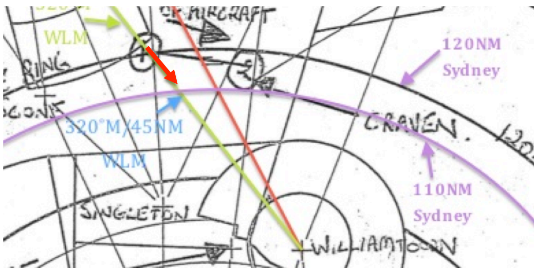
Figure 56: Overall track of 150°M. Readily seen is the overall progress of VH-MDX from the initial Sydney radar position to 320°M/46NM being close to 150° (Image: Australian Government (Department of Transport) 1981, additions Glenn Strkalj 2014).
