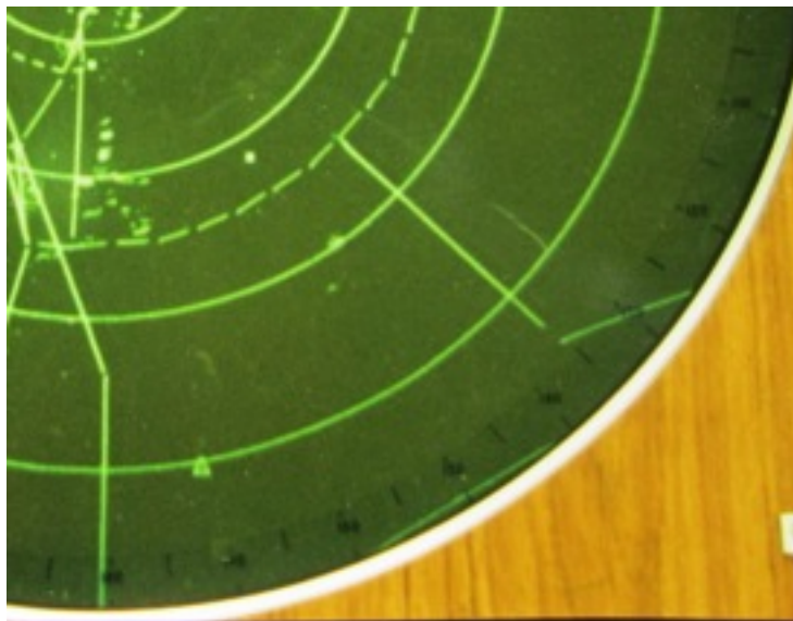
Figure 50: Williamstown SURAD approach PPI rose. This photo shows the compass rose with 5^\circ and 10^\circ marks and numeric values for each 10^\circ value. 10NM range rings are also visible. (Photo: H. Howard c.1983).
