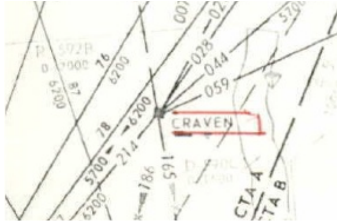
Figure 7: Craven intersection/waypoint. Craven waypoint is defined by bearings taken from at least two nav aids; not visual features. Magnetic bearings from Craven waypoint are included on the track lines to various nav aids. Taree NDB is on a bearing 059°M from Craven waypoint whilst West Maitland VOR is on a bearing 186°M from Craven waypoint. When these bearings are observed on each nav aid receiver then the aircraft is at Craven waypoint (Base image: Australian Government (Department of Transport) c.1981).
