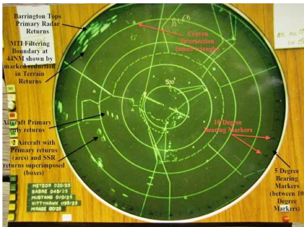
Figure 18: RAAF Williamtown Approach room SURAD PPI. North is at the top of the PPI. The compass rose on the circumference displays bearing in 10° increments with 5° markings in between. 10NM spaced rings are displayed to determine target range whilst airspace boundary markings and reporting points (small triangles) are also displayed. To the north-west from around 43NM are the Barrington Tops permanent echo terrain returns (Photo: H. Howard c.1983).
