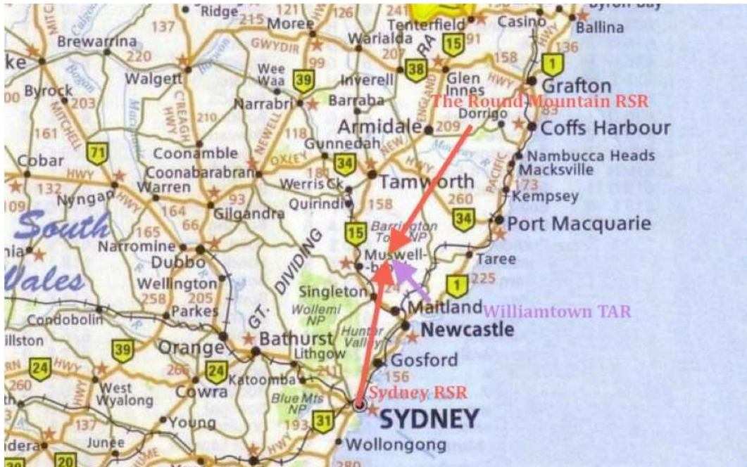
Figure 16: Relevant radar head locations. The Round Mountain RSR and Sydney RSR were operated by Sydney ATC (red arrows). Immediately obvious is how much closer to VH-MDX Williamstown TAR was. Despite this, only a single complete radar fix was obtained from the Williamstown TAR (Base Map: Melway Publishing Pty Ltd 2014, additions: Glenn Strkalj 2014).
