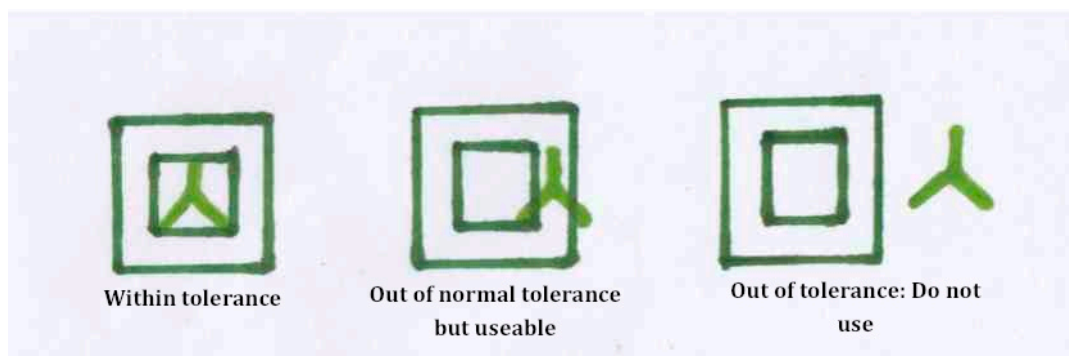
Figure 44: Northern Mosaic alignment markers (red circles). The ATCO would check if the illuminated inverted 'Y' was located within inner and outer boxes. Various levels of tolerance determined serviceability: This was only one of many calibration checks performed. Equipment was reportedly calibrated to very tight tolerances and there is no reason to suspect equipment was significantly out of tolerance during the VH-MDX accident. Despite this, it would be prudent to confirm calibration if applicable information ever presents. (Photo: M. Price c.1983, tolerance box drawing: Glenn Strkalj 2015).
