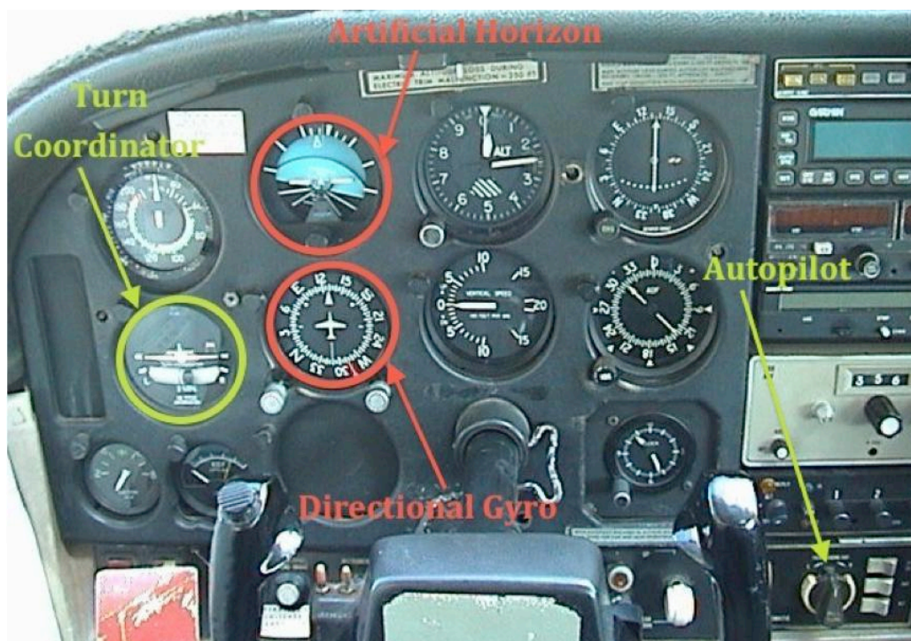
Figure 37: Cessna 210 instrument panel. Red = unserviceable, green = serviceable gyroscopic instruments. The AH and DG/DI were vacuum operated and were reported as unserviceable by the pilot of VH-MDX. The TC is electrically driven thus would have been serviceable. Autopilot roll error detection can be sourced from the DI for a 'heading select' type mode via the right knob on the DI or, from the TC for a 'turn-rate hold' type mode. Consequently, the pilot of VH-MDX had the ability to set a turn-rate and thus maintain a steady turn-rate or heading. Heading select was also still possible if the pilot continually, manually adjusted the DI for current compass heading. The autopilot shown is not the exact same model fitted to VH-MDX but, the 'pull-roll' knob is effectively the same (Photo: Glenn Strkalj 2002).
