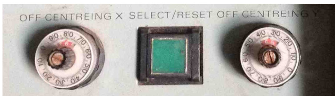
Figure 48: PPI offset controls. The displayed area on the PPI could be offset away from the radar head at origin position. This obviously changes the reference point for any bearing/range given so, the setting needs to be known in order to geographically plot radar fixes. Two controls were available to move the PPI origin position in both the X and Y-axis. The offset was then activated or cancelled by pressing the 'Select/Reset' button. Offset was confirmed as not being used during the VH-MDX accident thus, radar bearing/ range positions after modification for 1981 magnetic variation, can be directly plotted on charts. (Photo: Glenn Strkalj 2014, access to SURAD PPI courtesy of The Australian Aviation Heritage Centre).
