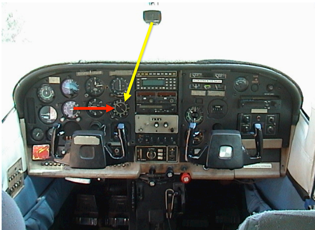
Figure 41: Bearing transposition onto the ADF. VH-MDX was likely fitted with a fixed card type ADF (located at the heads of the two arrows above) that displayed only relative bearings of the NDB to the aircraft. Pilots are required to mentally transpose heading information onto the relative bearing card of the ADF to yield magnetic bearings that are then useable for navigation. This is normally done by reference of the Direction Indicator (DI) positioned two instruments to the left of the ADF indicated by the origin of the red arrow. With the DI unserviceable, the pilot is forced to include the direct reading compass located at the top of the windscreen (indicated at origin of yellow arrow) into the scan that forces the pilot away from 'flying' the aircraft. Throw in the additional challenges of attempting to read the compass bouncing around in turbulence at night and it can be seen that maintenance of accurate NDB bearings is very challenging (Photo: Glenn Strkalj 2002).
